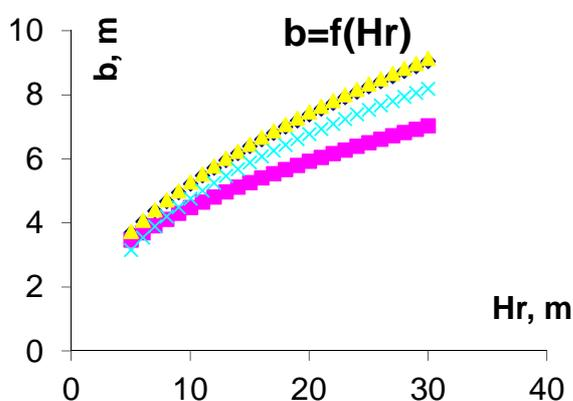
This sample of about fifteen Algerian dams was used as work base knowing that the top width is closely linked to the embankment height, as shown by the sample. The four (04) formulas have allowed, based on approaches more or less logic, searching for the consensus between them. This consensual approach allowed determining six (06) mathematical relations.
