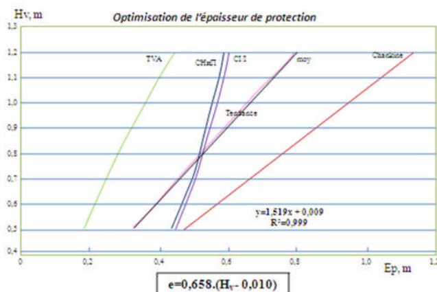
Once the lower and higher bounds of ranges are defined, we have carried out a dimensional analysis in order to determine the law to which belongs the intermediary curve to stress the optimum relation of embankment protection.
