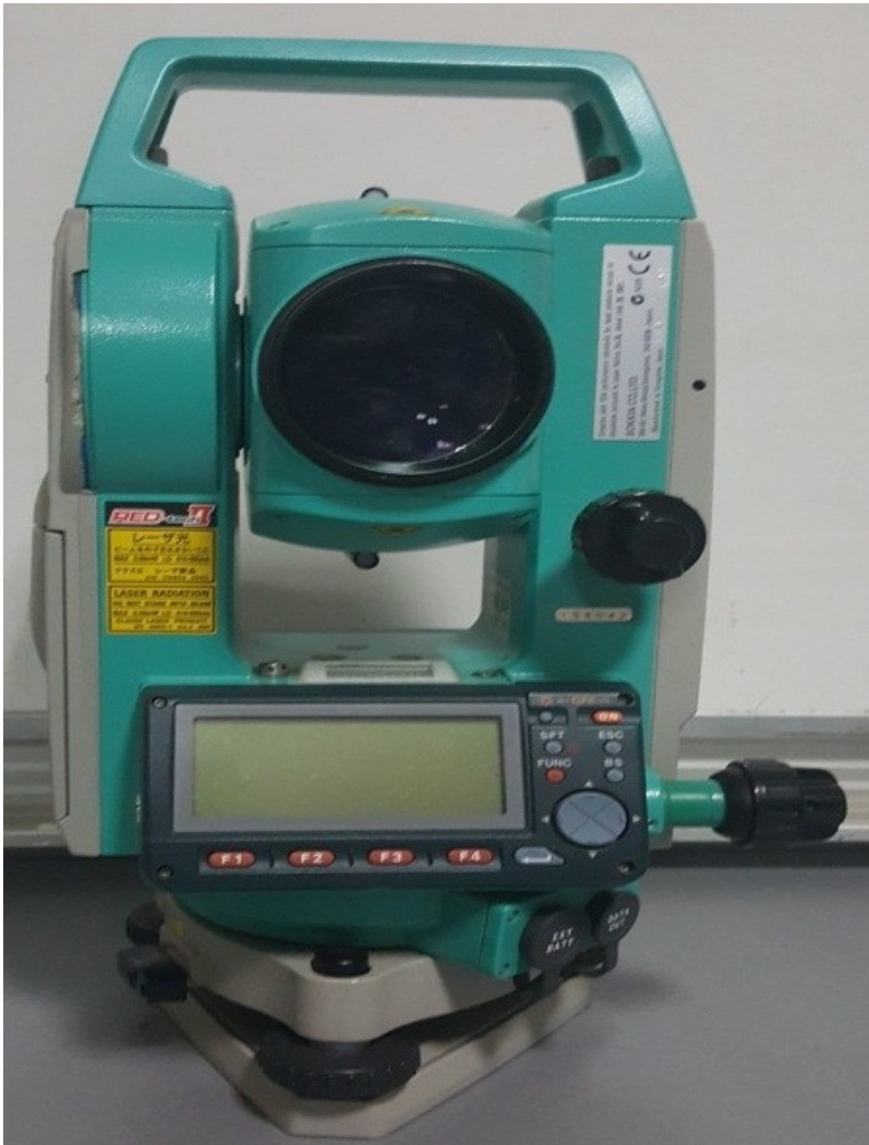
DIAZOMETRIE STATION TOTALE SET 5300 mètres (prisme triple), faisceau laser coaxial visible, m
