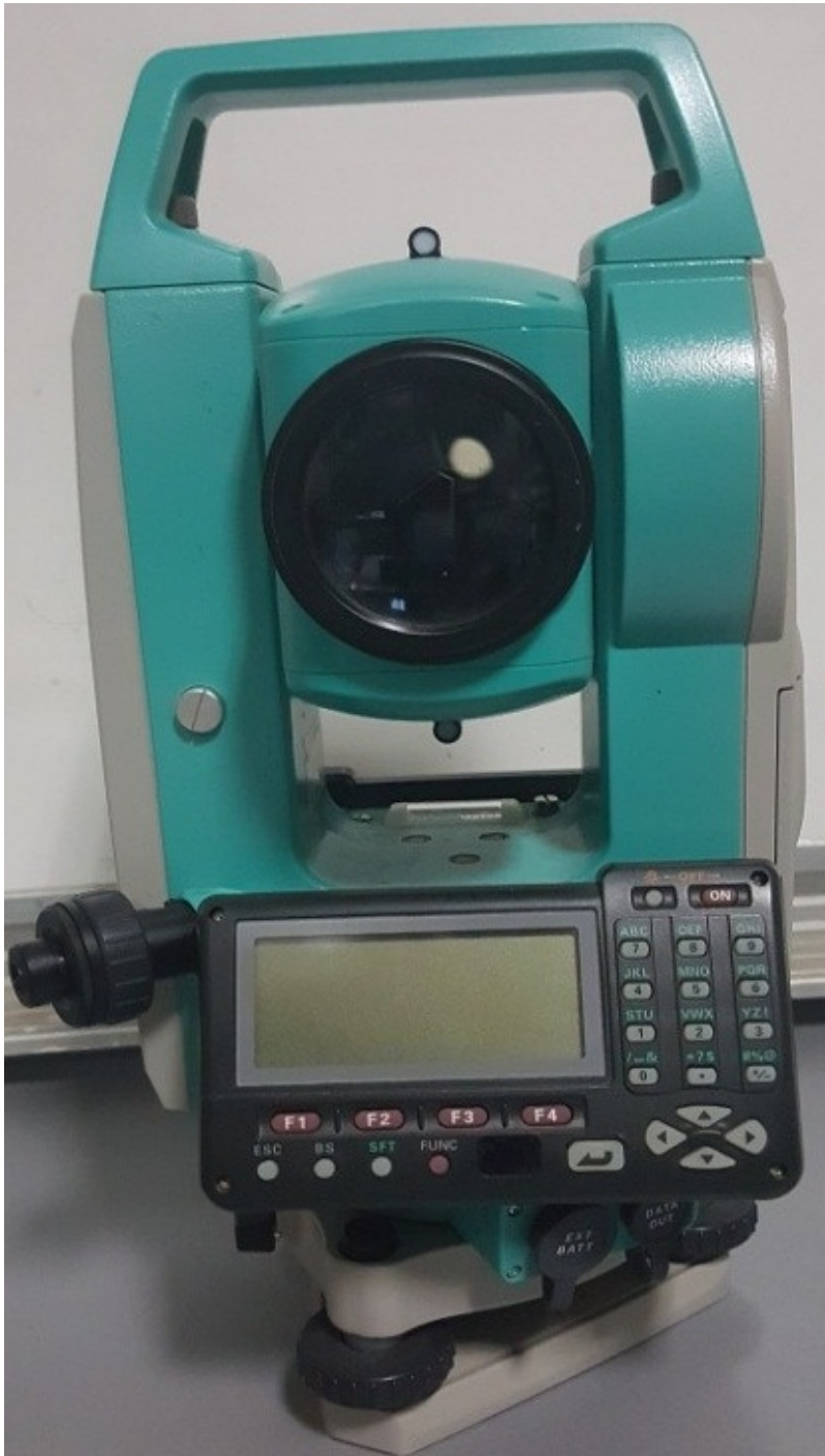
Station Sokkia SET 520K (prisme triple), faisceau laser coaxial visible, m
